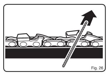
Put a few firm strokes on every tooth. File all left hand cutters in one direction. Then move to the other side and file the right hand cutters in the opposite direction. Occasionally remove filings from the file with a wire brush.
